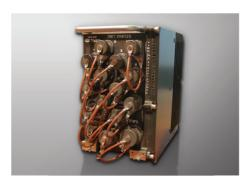
ATR is a standard that specifies form fit and function of a "black box" installed in the aircraft. This standard also known as ARINC and was designated as ARINC 404 standard.
