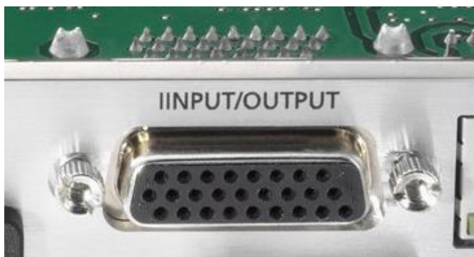
Figure 3-11: High density SUB-D DIO connector 26 Pol
