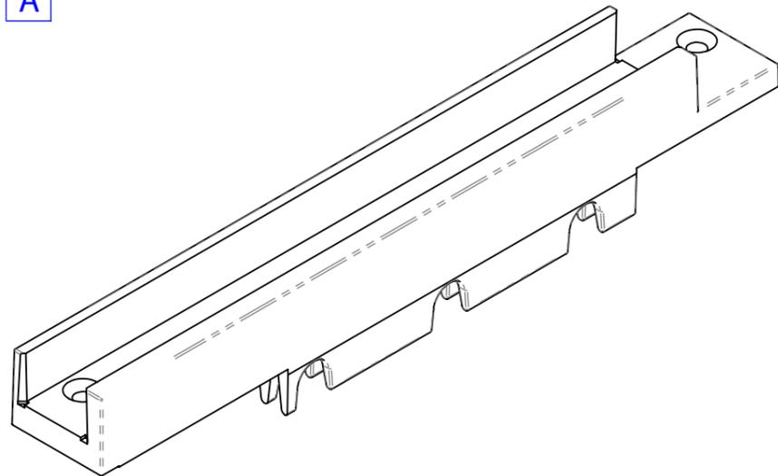
The kit p/n C201.10684 consists of two conduction cooled guide rails and 4 screws
