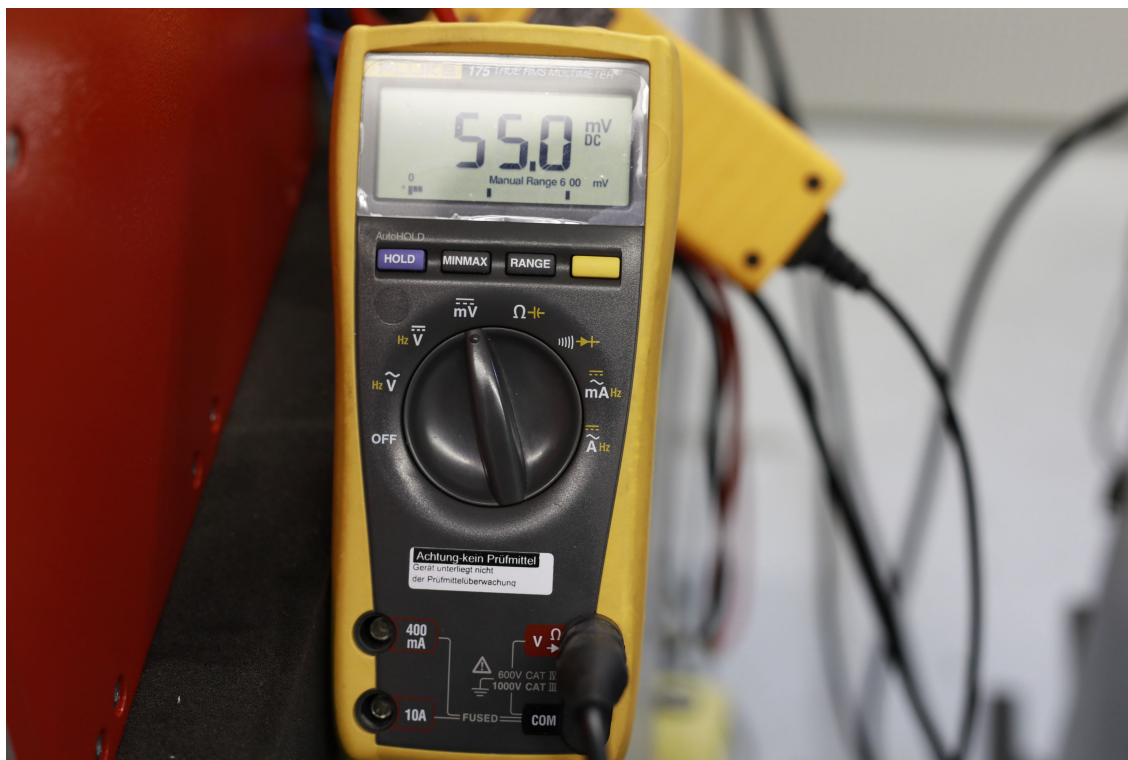
Image 7.6: Functional test after vibration test
